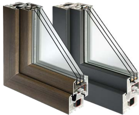
Kombisystem / Kombisystem Alu 6 chamber system, construction depth: 83 mm. Aluminum cladding. Triple gasket system. Available also with optional external aluminum cladding.
