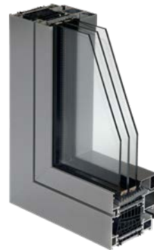
MB 104 Construction depth 95 mm. Passive house certified product, U_w from 0.53 W / m 2 K.
